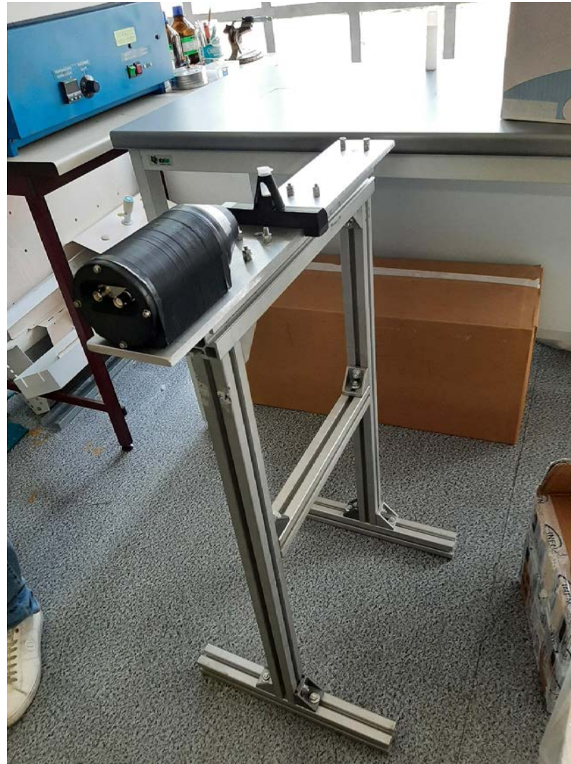
LBC 1"x1" LBC-based \gamma -counter with a 3D printed vial holder
