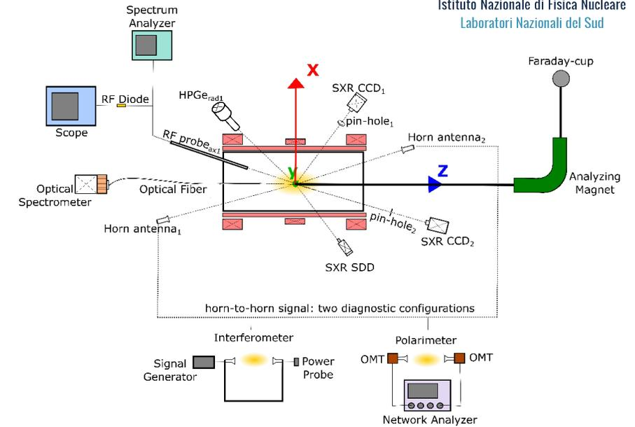
SDD for "warm electrons": probing volumetric soft X-radiation (2 – 20 keV)
