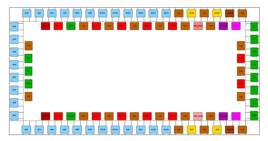
Final Pad Ring => 94 pads (52 in the outer ring, 42 in the innr ring) PWR/GND => 25 GND, 2VDD\_IO, 2 VDD\_HSIIO, 2VDD\_BIST, 12 VDD\_SER) Signals => 12 LVDS I/O, 4 LVDS\_IN, 1 CML IN, 1 CML OUT, 13 Analog I/O
