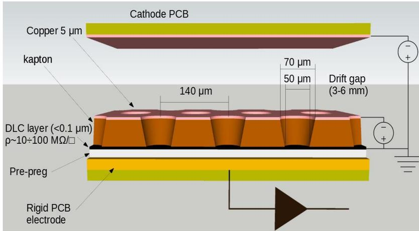
The  $\mu$ -RWELL is a resistive MPGD composed of two elements:
