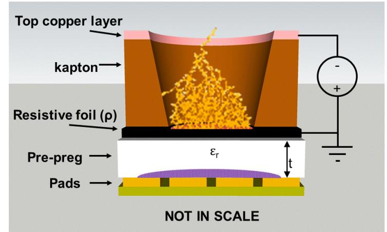
The “WELL” acts as a **multiplication channel** for the ionization produced in the drift gas gap.
