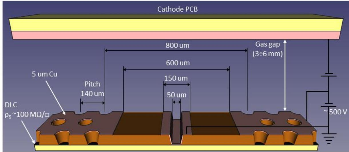
The PEP layout (Patterning – Etching – Plating) is the state of art of the high rate layout of the  $\mu$ -RWELL
