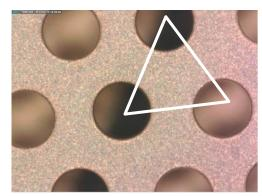
Dielectric Thickness: 400 µm Hole Ø: 400 µm Hole in triangular pattern Hole pitch: 800 µm No rim
