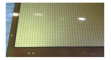
Readout pad size: 7.5 x 7.5  $mm^2$ Readout pad pitch: 8 mm
