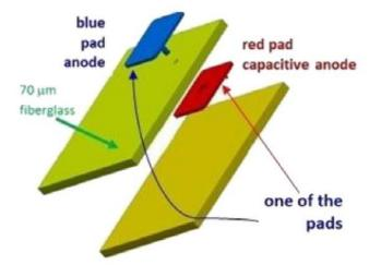
"resistive" MM: 470 M $\Omega$  in series with each pad Signal collected by buried pad and read with APV25 chip
