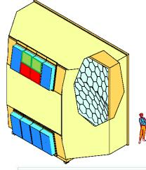
Cover large area with photon detectors in COMPASS RICH (~1.4  $m^2$ )
