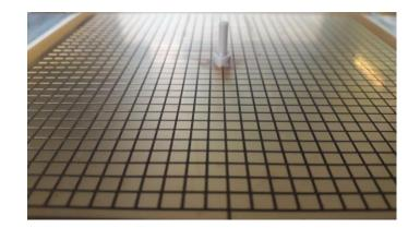
Reduced readout pad size ( $3x3 mm^2$ )
