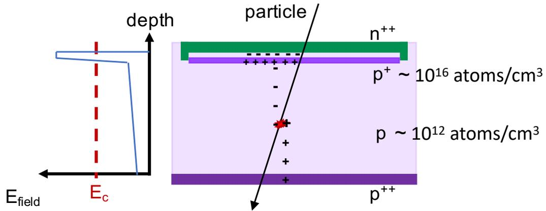
The acceptor removal mechanism deactivates the  $p^+$ -doping of the **gain layer** with irradiation according to
