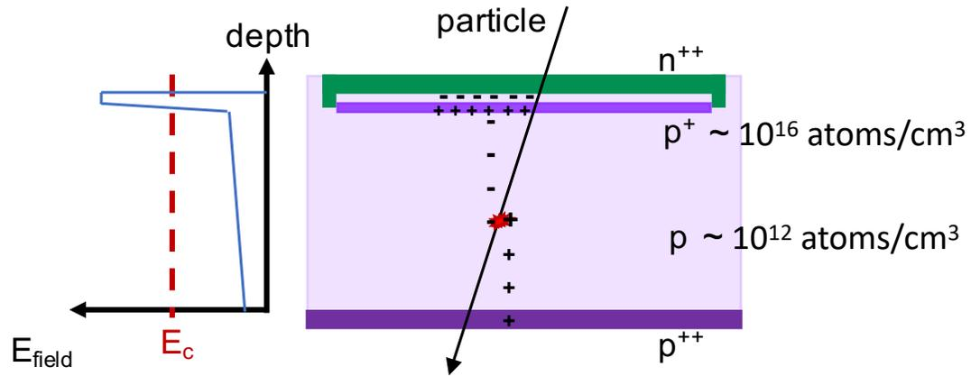
Low-Gain Avalanche Diodes (**LGADs**) are n-in-p silicon sensors
