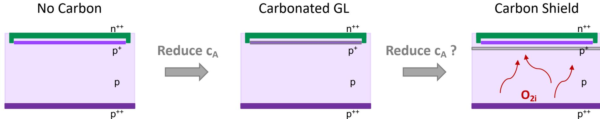
A spray of Carbon will be introduced below the gain layer region to protect the gain layer atoms from defects moving towards the  $n^{++}$  electrode during process thermal loads or exposure to particle radiation
