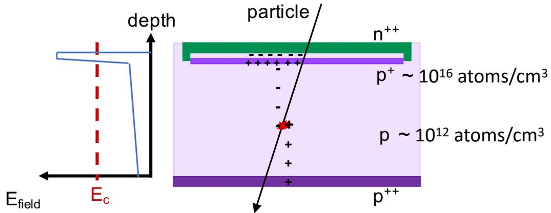
The acceptor removal mechanism deactivates the p<sup>+</sup>-doping of the **gain layer** with irradiation according to
