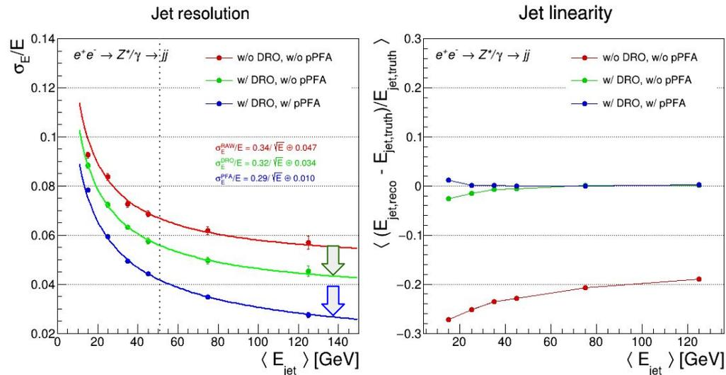
**Sensible improvement in jet resolution using dual-readout information combined with a particle flow approach  $\rightarrow$  3-4% for jet energies above 50 GeV**
