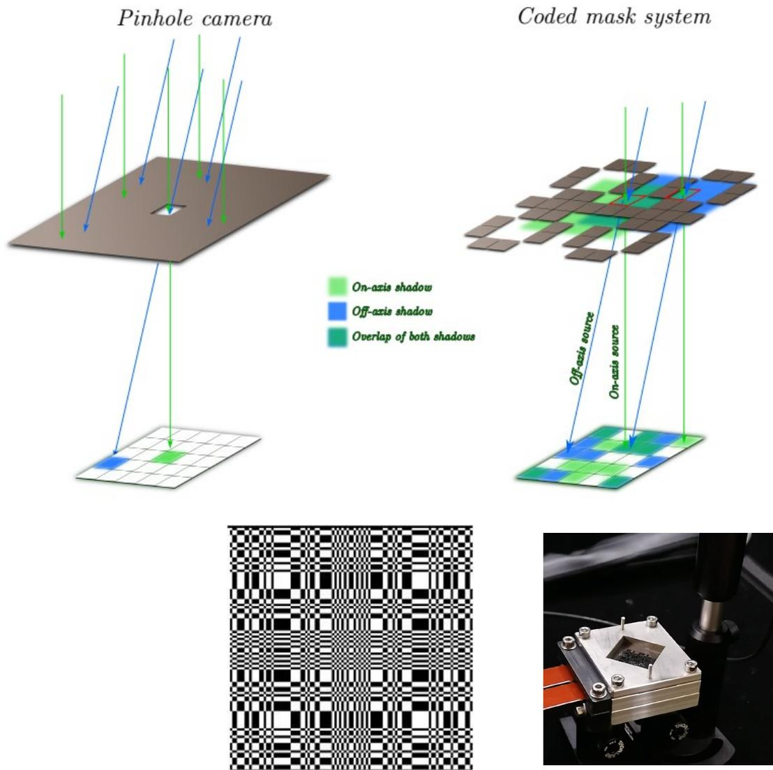
Coded aperture mask techniques were developed as the evolution of a single pinhole camera
