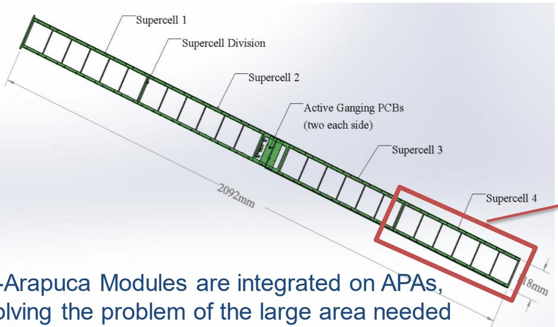
X-Arapuca Modules are integrated on APAs, solving the problem of the large area needed (10 modules x APA)
