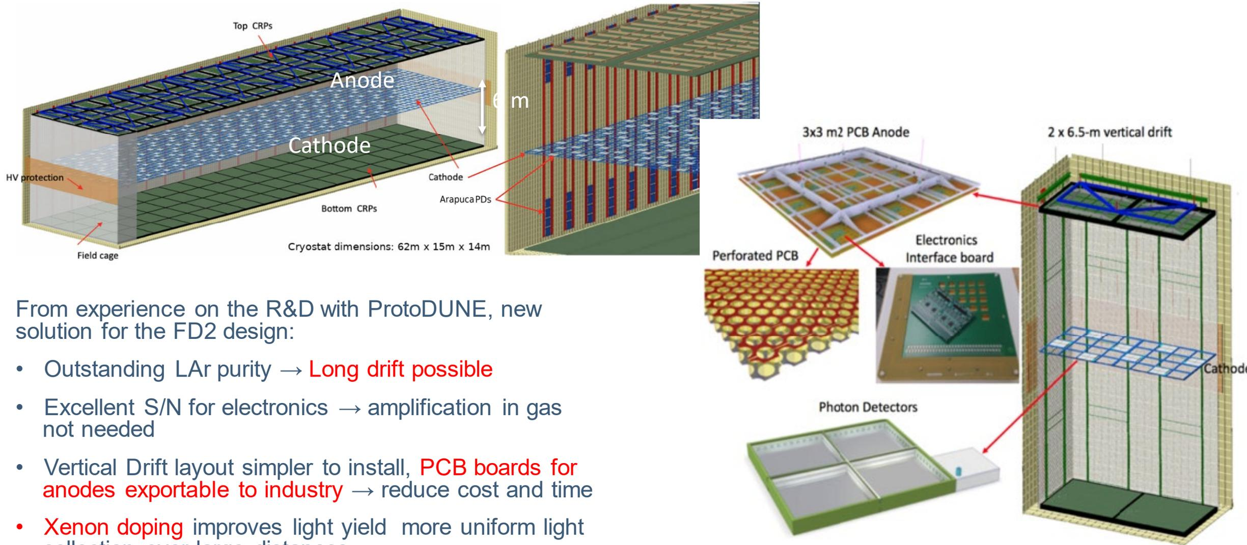
From experience on the R&D with ProtoDUNE, new solution for the FD2 design:
