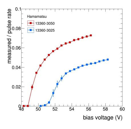
the LED setup can measure differences in the PDE between 50 and 25 um Hamamatsu sensors
