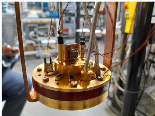
Left: Chip bonded on the sample holder. Right: Sample holder mounted in the dilution fridge at Laboratori Nazionali di Frascati (LNF)
