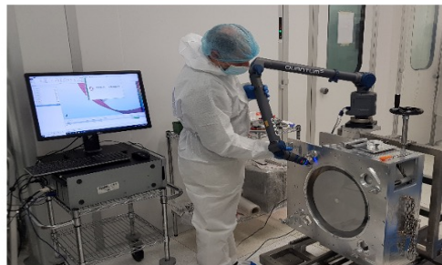
HCB procedure at LMA and at positioning test with FARO arm Virgo/EGO site
