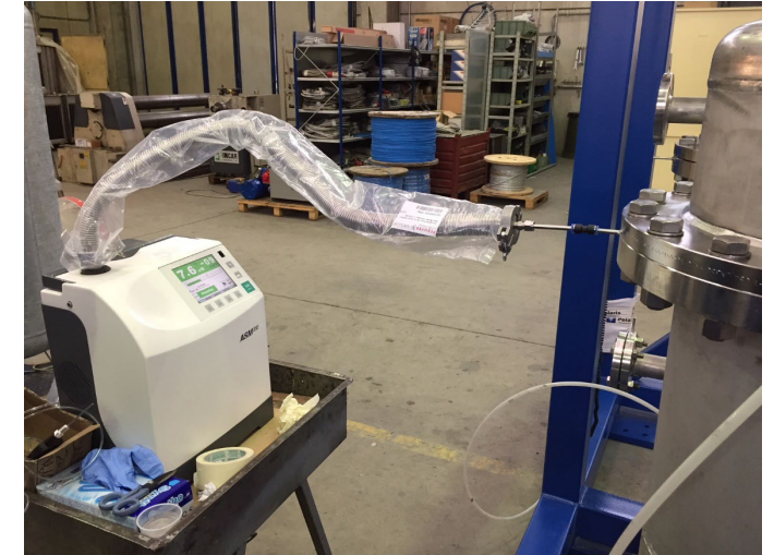
Leak detector for flange tightness certification
