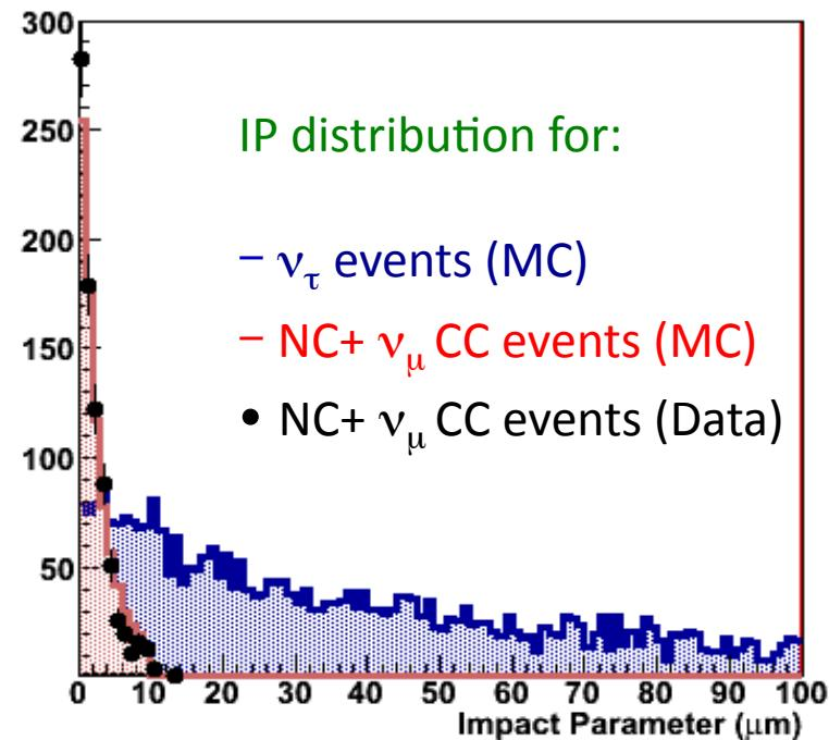
The detection of decay topologies is triggered by the observation of a track with a large IP wrt the primary vertex, in addition to kink detection.
