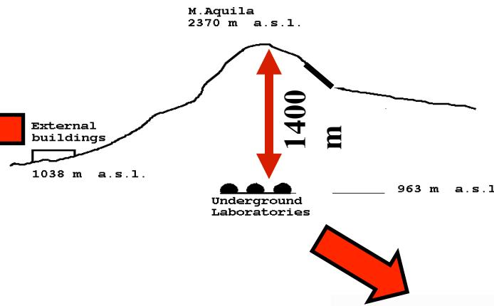
Gran Sasso underground lab: 1400 m of rock (3800 m.w.e) shielding, cosmic ray flux reduced by a factor  $10^6$  w.r.t. surface, very reduced environmental radioactivity.
