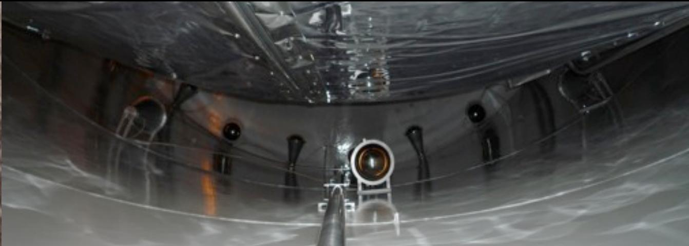
Inner-Veto Detector (scintillator)  $\Rightarrow$  tag  $\mu$ s & possibly fast-neutrons
