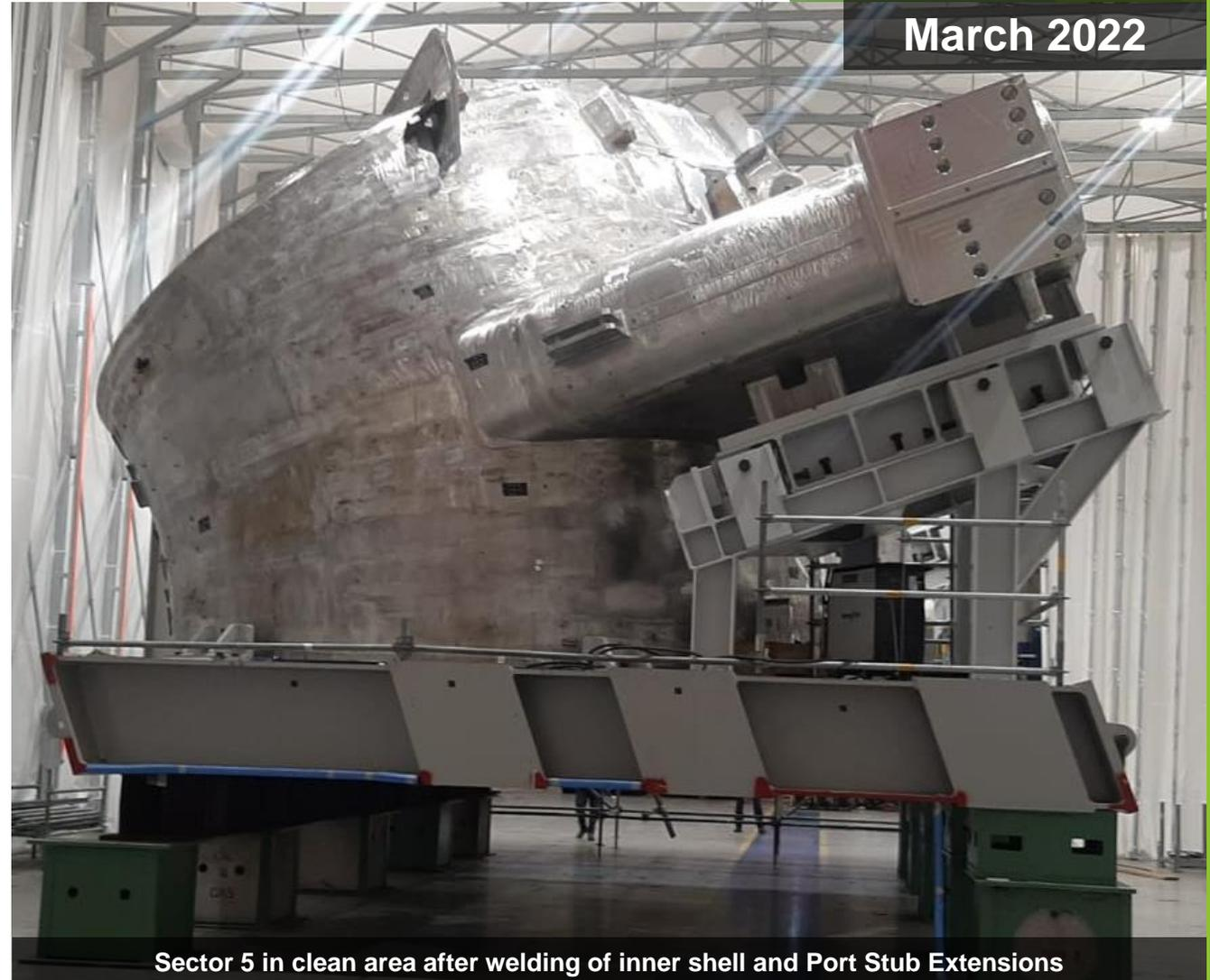
Sector 5 in clean area after welding of inner shell and Port Stub Extensions
