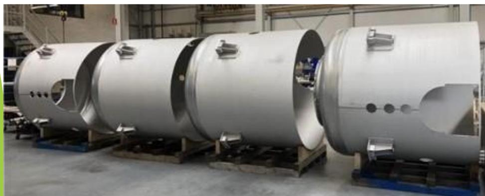
1<sup>st</sup> batch of 4 CVB vacuum chambers manufactured
