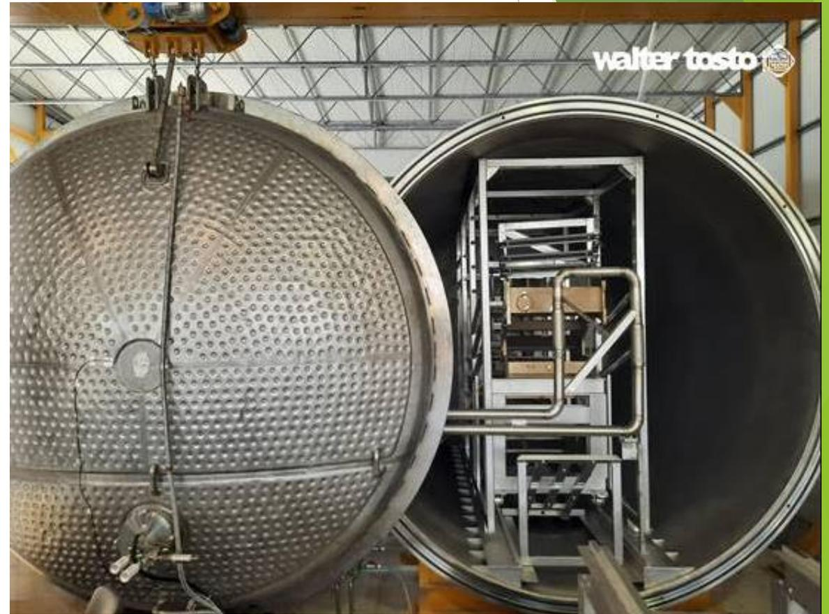
Commissioning of Hot Helium Leak test facility at Walter Tosto (Italy)
