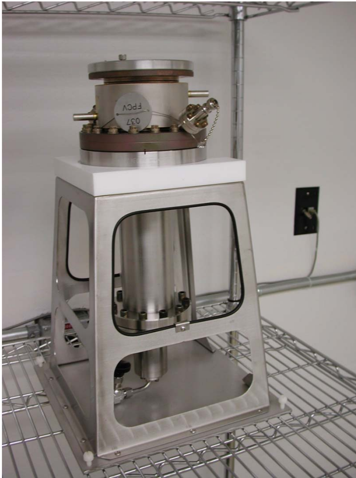
Storage on outer conductor using protection cup, under dry dust free nitrogen.
