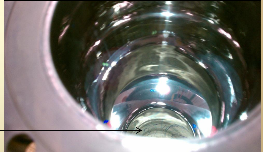
Single Cell Polished to Mirror Finish
