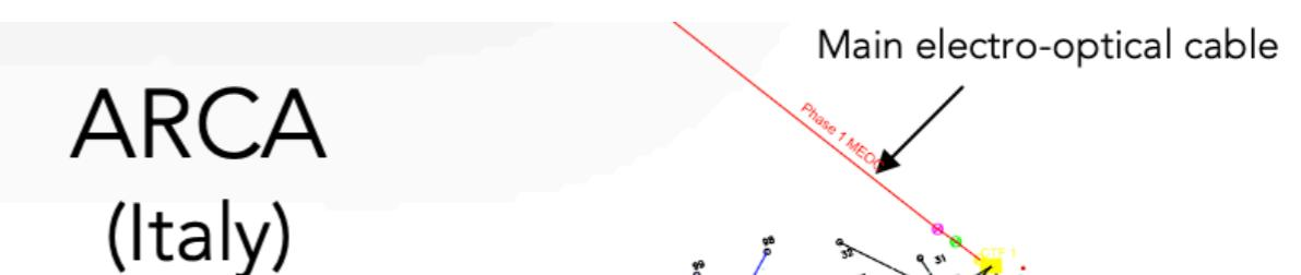
**ARCA** is composed of 2 building blocks of 115 DUs each with 90 m DU interspacing and 36m inter DOM spacing (Total Volume  $\sim 1 \text{ km}^3$ )
