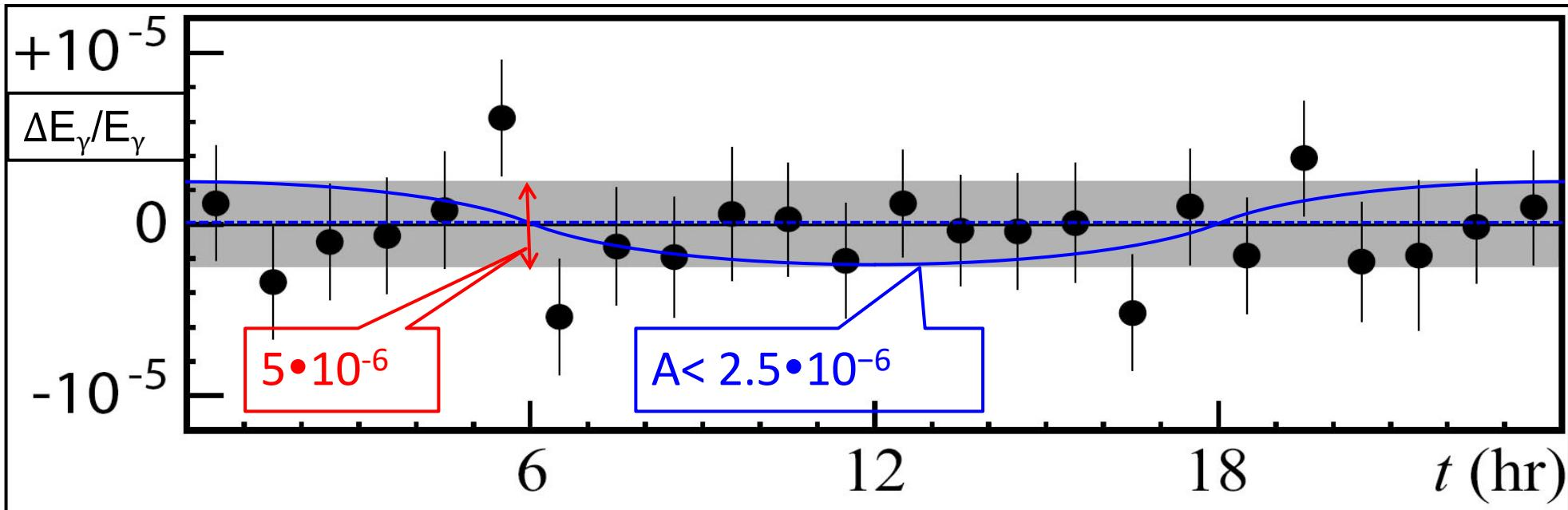
14765 CE spectra grouped in 24 bins, with about 600 measurements each, corresponding to the hours of the sidereal day and averaged. The error bars are purely statistical and agree with the dispersion of the data points ( $\chi^2 = 1.04$  for the unbinned histogram). The blue line is a fit of the form:  $A \sin(\Omega t + \varphi)$ . [ $\Omega \approx 2\pi/(23 \text{ h } 56 \text{ min})$ ] and at 95% Confidence Level yields:
