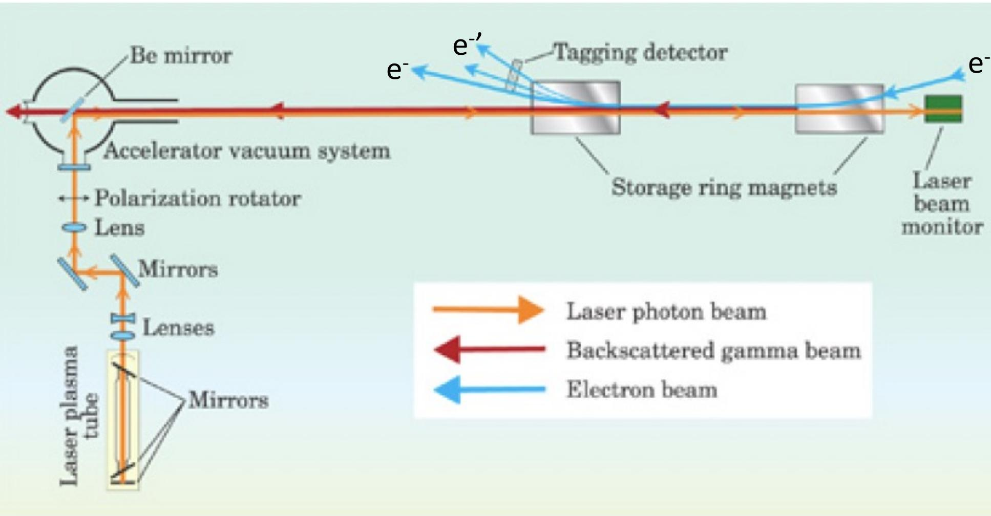
Scattering of polarized Laser photons on ultra-relativistic electrons in a storage ring
