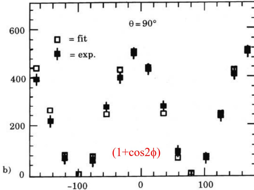
The first verification of the polarization of Ladon beams was performed at Frascati with the elastic scattering of the Ladon gamma-ray beam on the **15.1 MeV level of  $^{12}\text{C}$**  using the small NaI crystal ball ( $7_\theta \times 16_\phi$ ) of the University of Rome "La Sapienza". The experimental points reproduce very well the  $(1+\cos 2\phi)$  law expected for a fully polarized beam on a perfect polarization analyzer.
