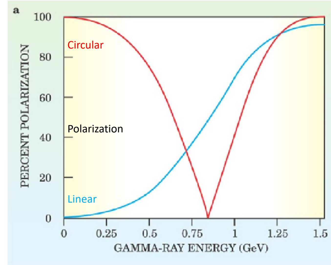
The calculated fractional polarization of the gamma-ray beam at the **Graal** facility, as a function of energy. The red and blue curves indicate, respectively, circular (absolute value) and linear polarizations.
