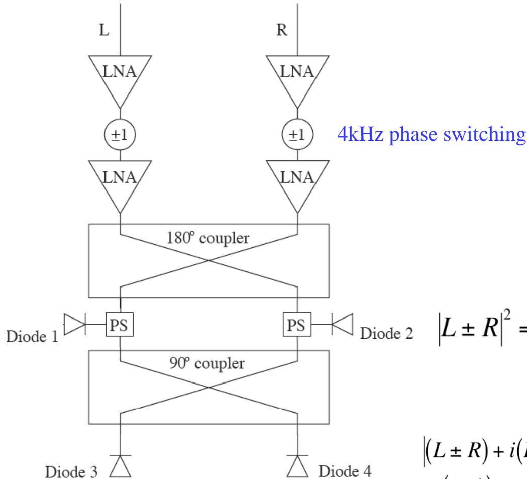
Differencing of phase-switched data streams at 4kHz and 50Hz protects against various instrumental systematics
