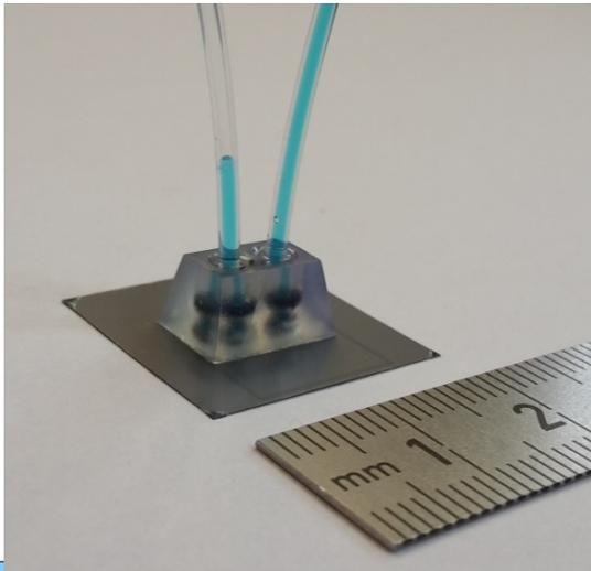
*Working MALTA CMOS sensor with integrated μ-channels*
