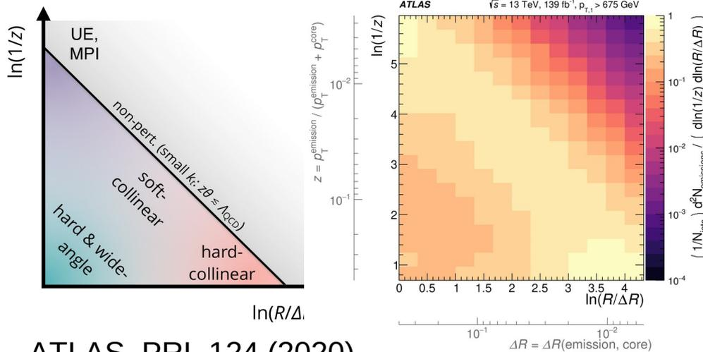
The Lund jet plane provides an image of the jet that separates hard splittings (matrix element), soft and collinear radiation (parton shower) and non-perturbative effects (hadronization model)
