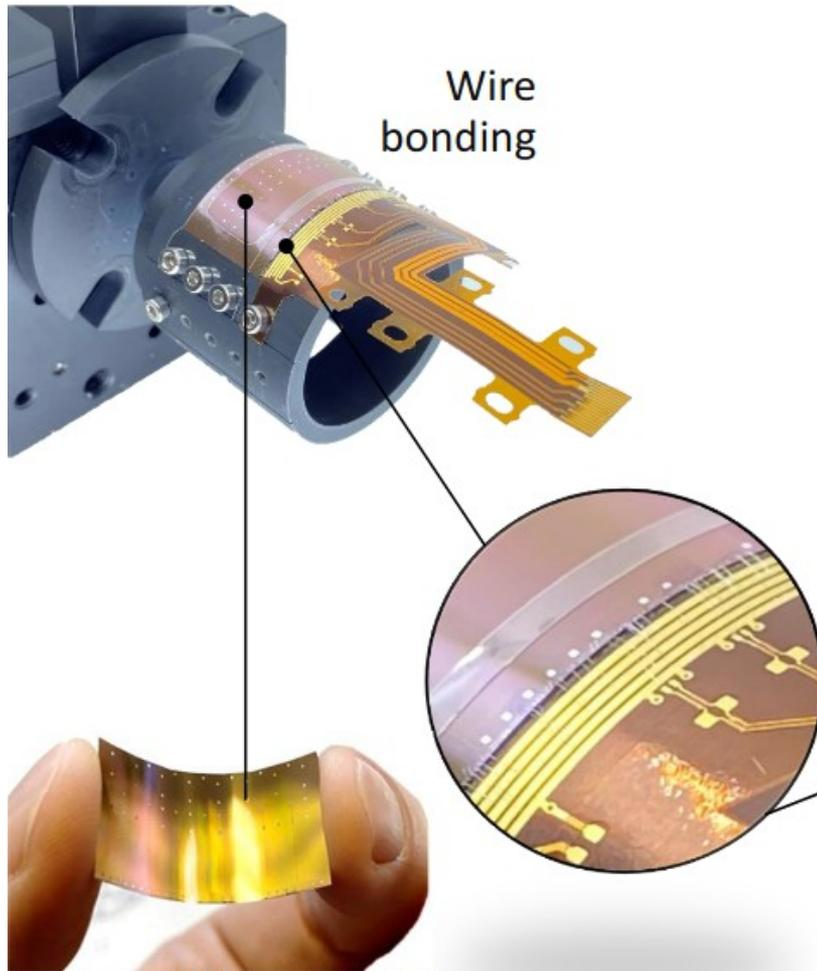
The Mu3e experiment and ALICE have aggressive plans to reduce detector material (Kapton support structures, bent sensors)
