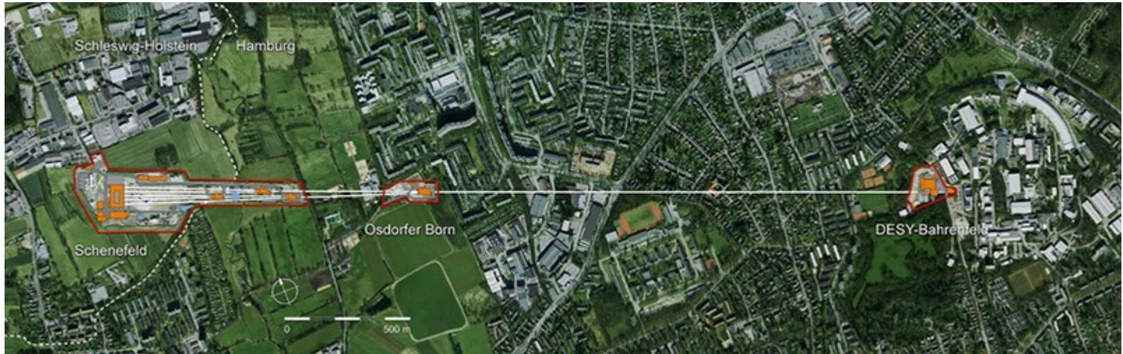
European XFEL at DESY Hamburg is a 19.5 GeV linear accelerator that is used to generate energetic X-ray beams for “photon science”
