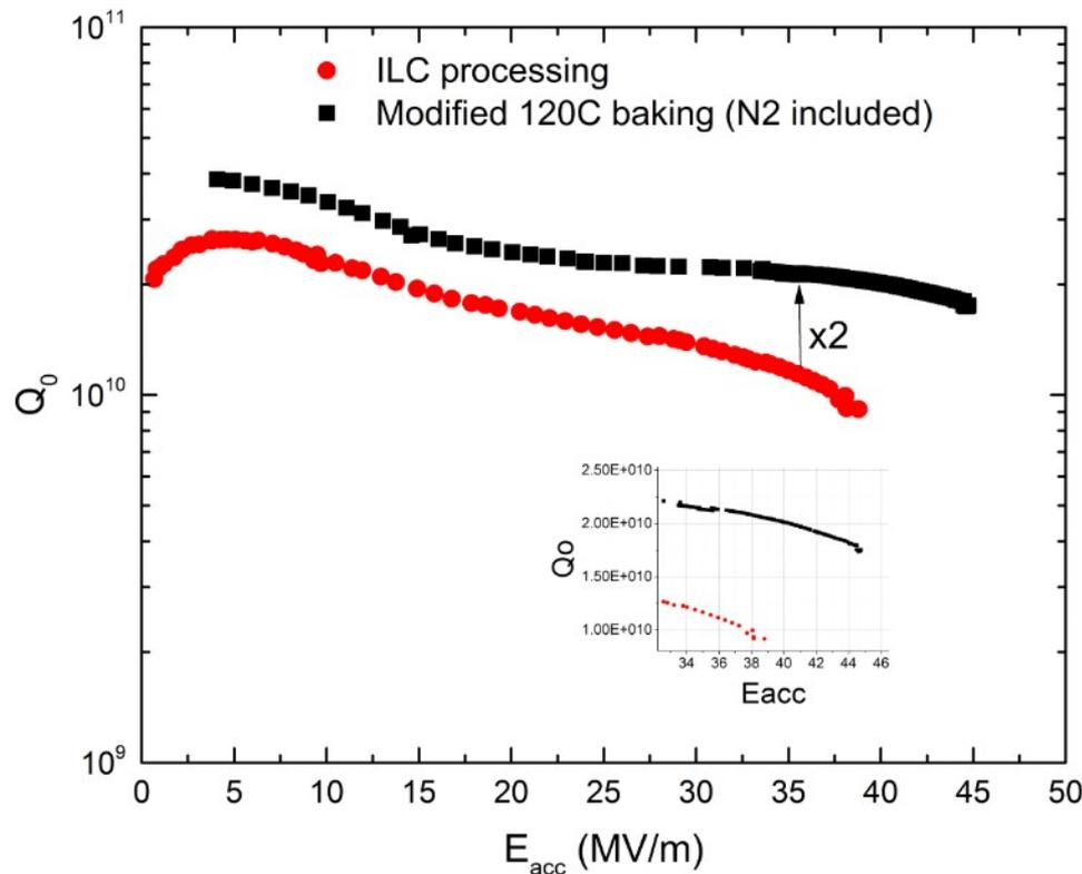
\* $Q_0$  quality factor that is inversely proportional to the surface resistance and power dissipation in the cavity walls
