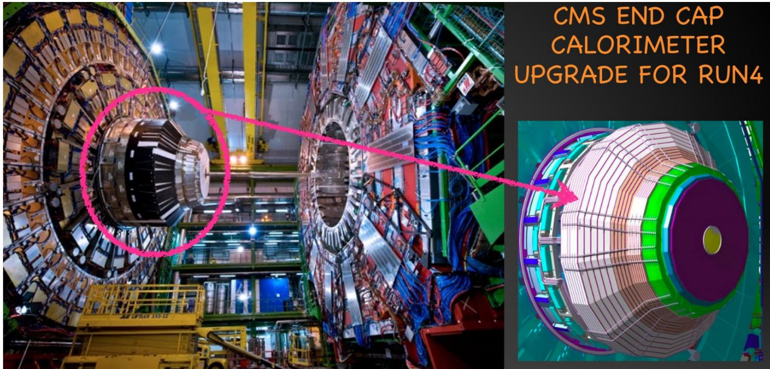
CMS HGCal, a complete Si+absorber sampling calorimeter prototype, Solidly establishes the ultra-granular “CALICE-style” calorimeters as the baseline for ILC (both ILD and SiD)
