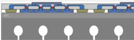
XeF<sub>2</sub> etching of microchannels (isotropic)
