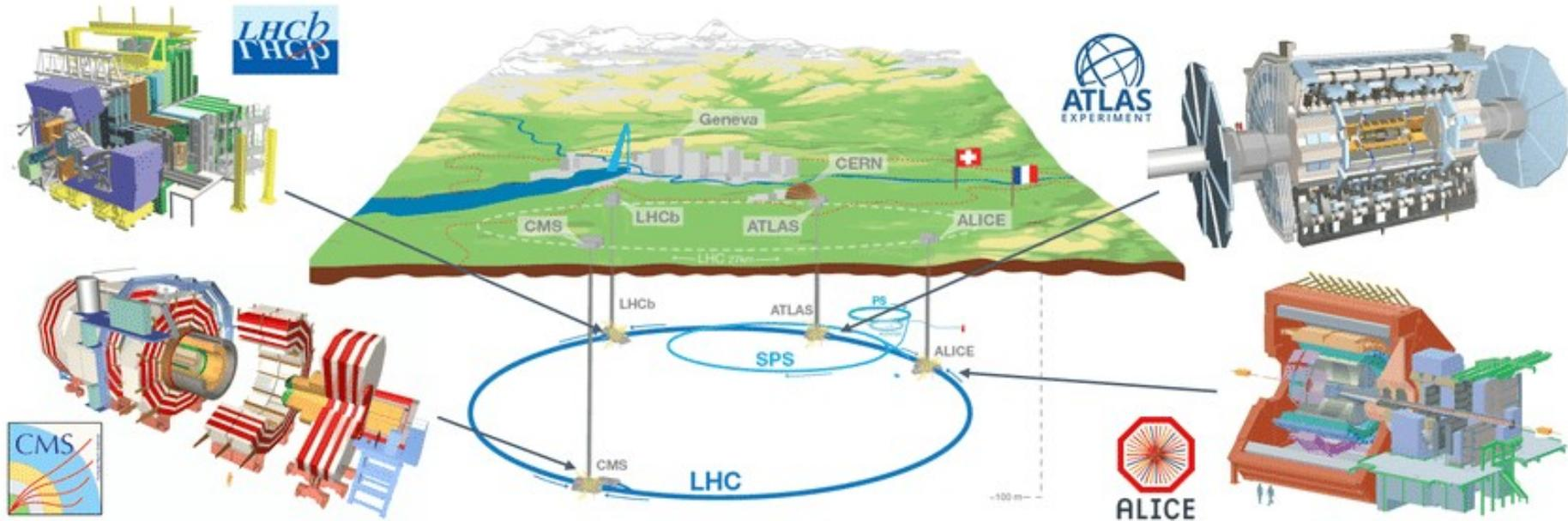
Beams cross and collide at 4 interaction points, equipped with experiments that register the products of the collisions
