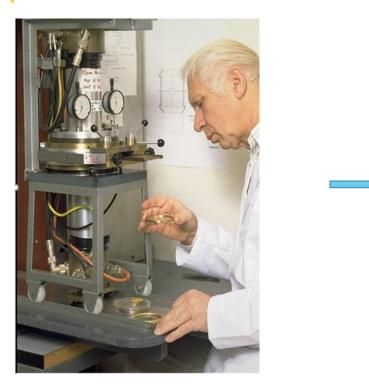
Above: The CsI detector at JRC-Geel on which part of the international reference system for radioactivity relies
