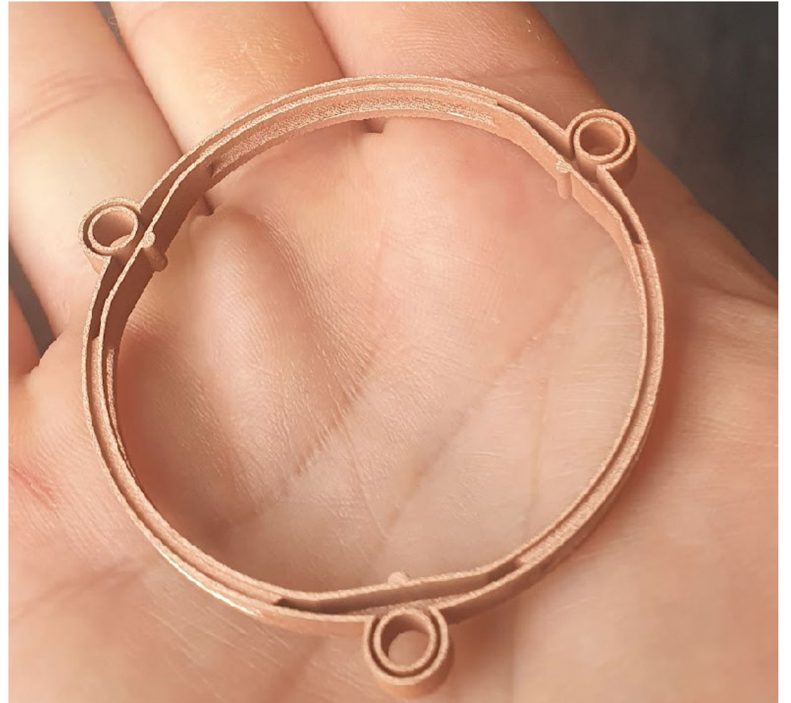
Low weight frame for Bolometric light detector (CUPID-0 R&D)
