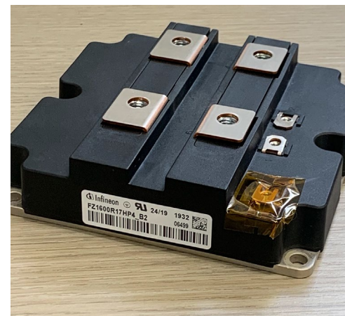
IGBT substitution after fault
