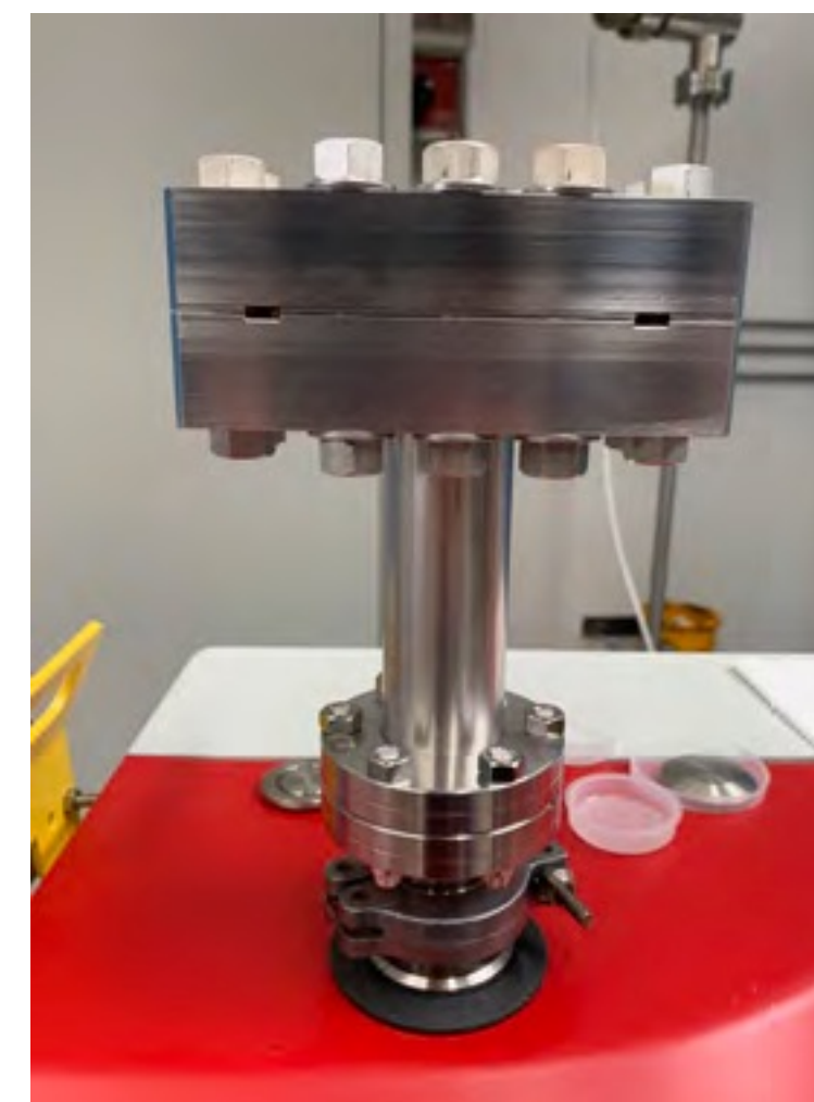
Setup for the thermal and vacuum leak tests
