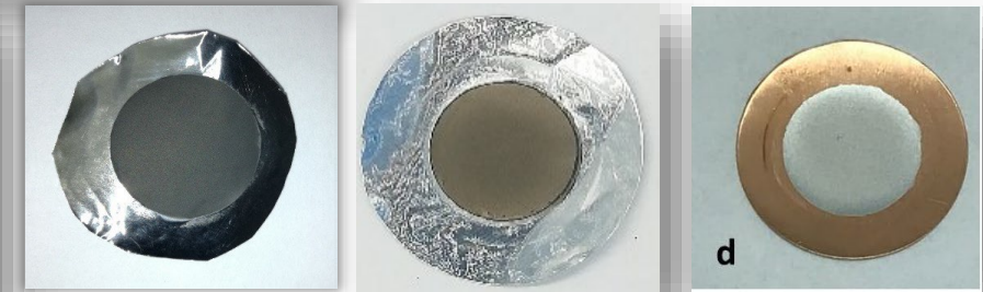
^{48}\text{Ti} (left) and ^{49}\text{Ti} (right) deposited (0.2–2 \text{mg}/\text{cm}^2 ) on Al foil (25 \mu\text{m} ) \text{natMo} on Cu foil (250 \mu\text{m} )
