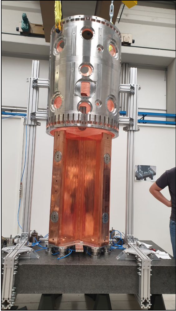
Initial positioning of the tank vs electrodes in vertical position
