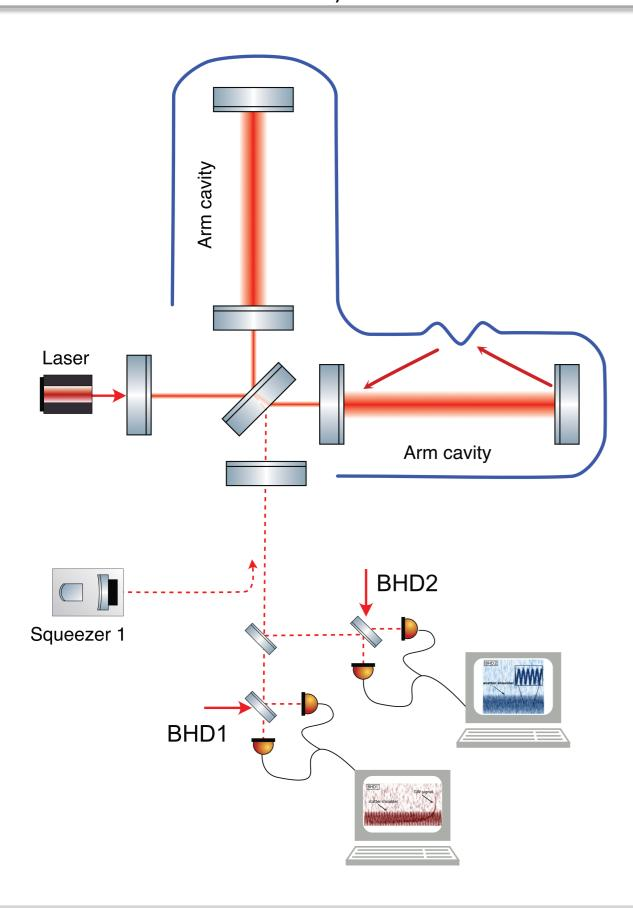
Squeezed light allows to reduce the shot noise in Y quadrature
