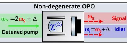
The interferometer itself acts like a detuned filter cavity for the idler! **Idler** experiences FDS
