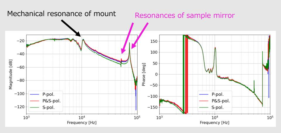
Electric field also couples through mechanical motion.
