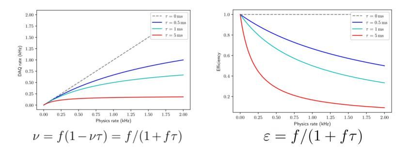
In modern experiments (e.g. FOOT) the event receiving is completely **decoupled** from data processing to absorb input rate fluctuations (this is why we have busy, timestamps etc.)
