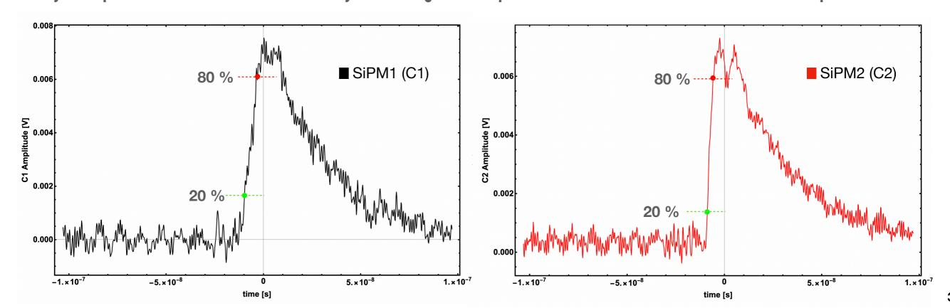
Timing properties of the system composed of two orthogonal scintillating bars 10 & 13 embedded in the prototype tested at CERN
