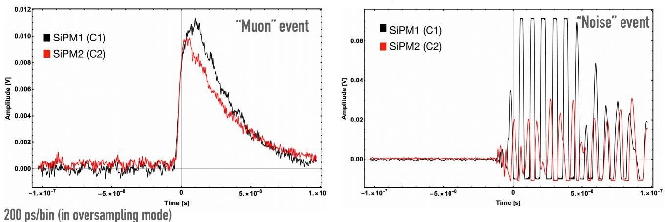
The analysis is performed at the waveform level by measuring relevant parameters (Rise Time (i.e. 20%–80%), Max Amplitude, Baseline)
