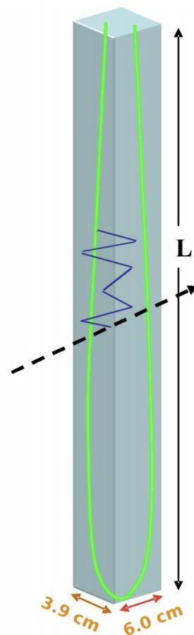
Low Z tracking calorimeter composed of alternating horizontal and vertical planes of liquid scintillator filled cells.
