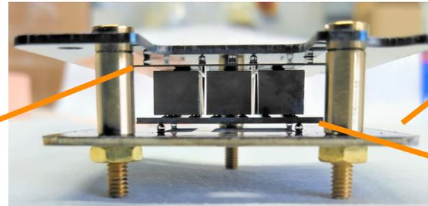
Inner detector module: side view
