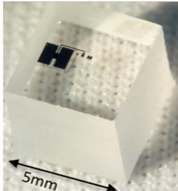
5mm-cube of  $\text{Al}_2\text{O}_3$  or  $\text{CaWO}_4$
