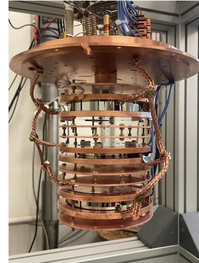
2x cyl. crystals during cryogenic performance test
