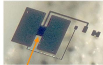
superconducting tungsten film
