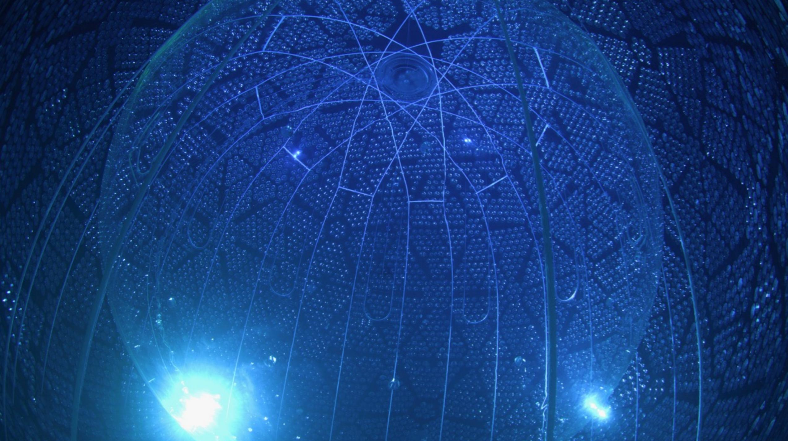
Main detector body is 6m radius acrylic vessel
