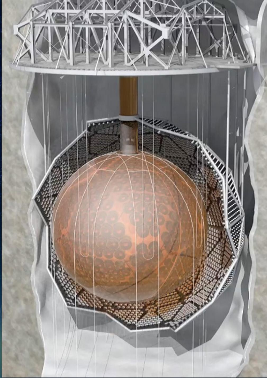
System of low-radioactivity external ropes to account for buoyancy differences between various media
