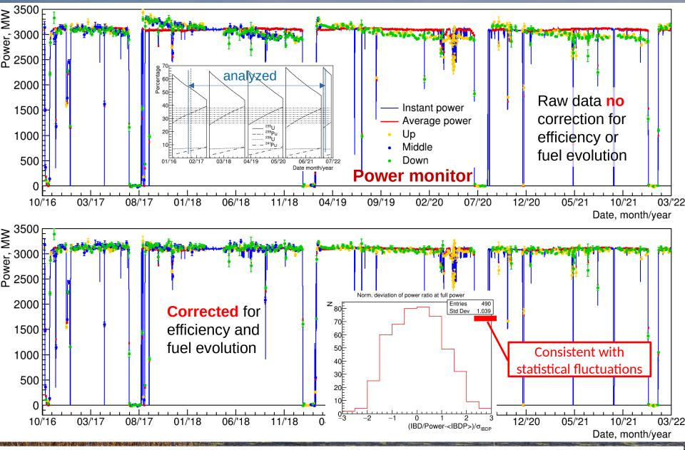
Reactor power is measured by neutrino flux with 1.5% statistical accuracy in 2 days for 5.5+ years. Changes in absolute detector efficiency are known with accuracy better than 1% during 5.5+ years. Relative efficiency is even more stable (<0.2%) because of frequent changes of detector positions.
