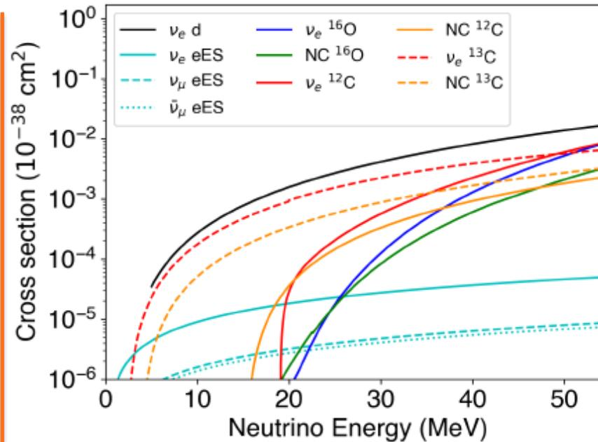
Neutrino-electron scattering background is insignificant because of low cross section
