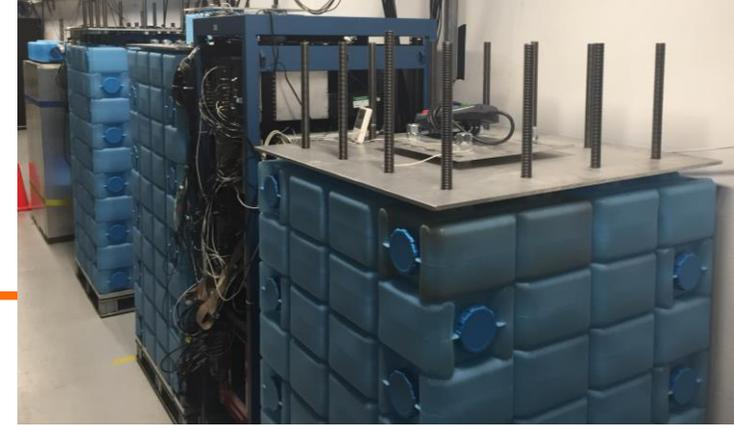
Nubes was a liquid scintillator detector that observed NINs (neutrino induced neutrons), via inelastic scattering.
