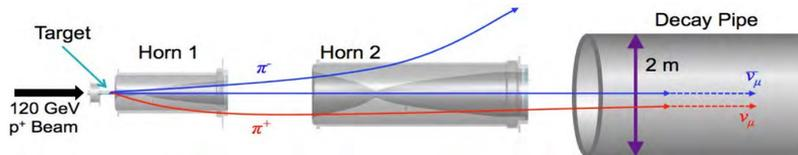
Horn-focused neutrino beam line optimized for CP violation sensitivity using genetic algorithm
