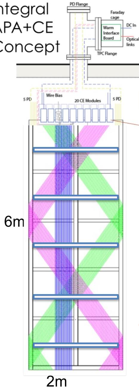
**Core detector element: Anode Plane Assemblies (APA) with integrated Cold Electronics Boards and Ph.Detector modules**
