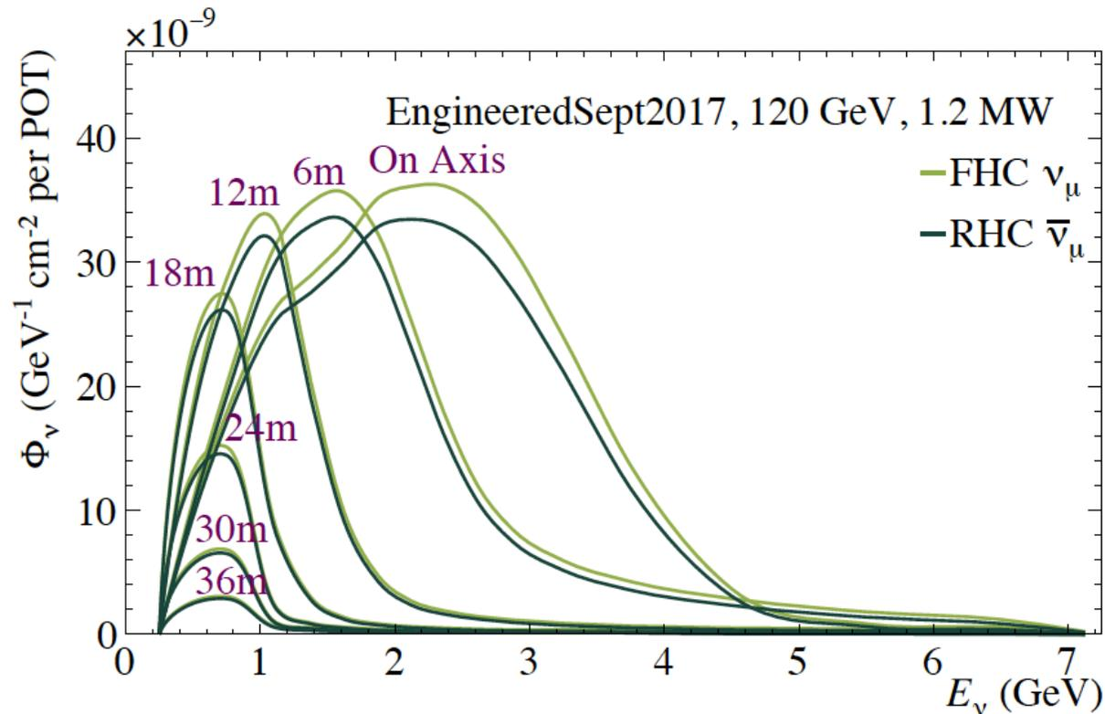
Capability to move ND (LAr+TMS) for off-axis measurements (DUNE-Prism)
