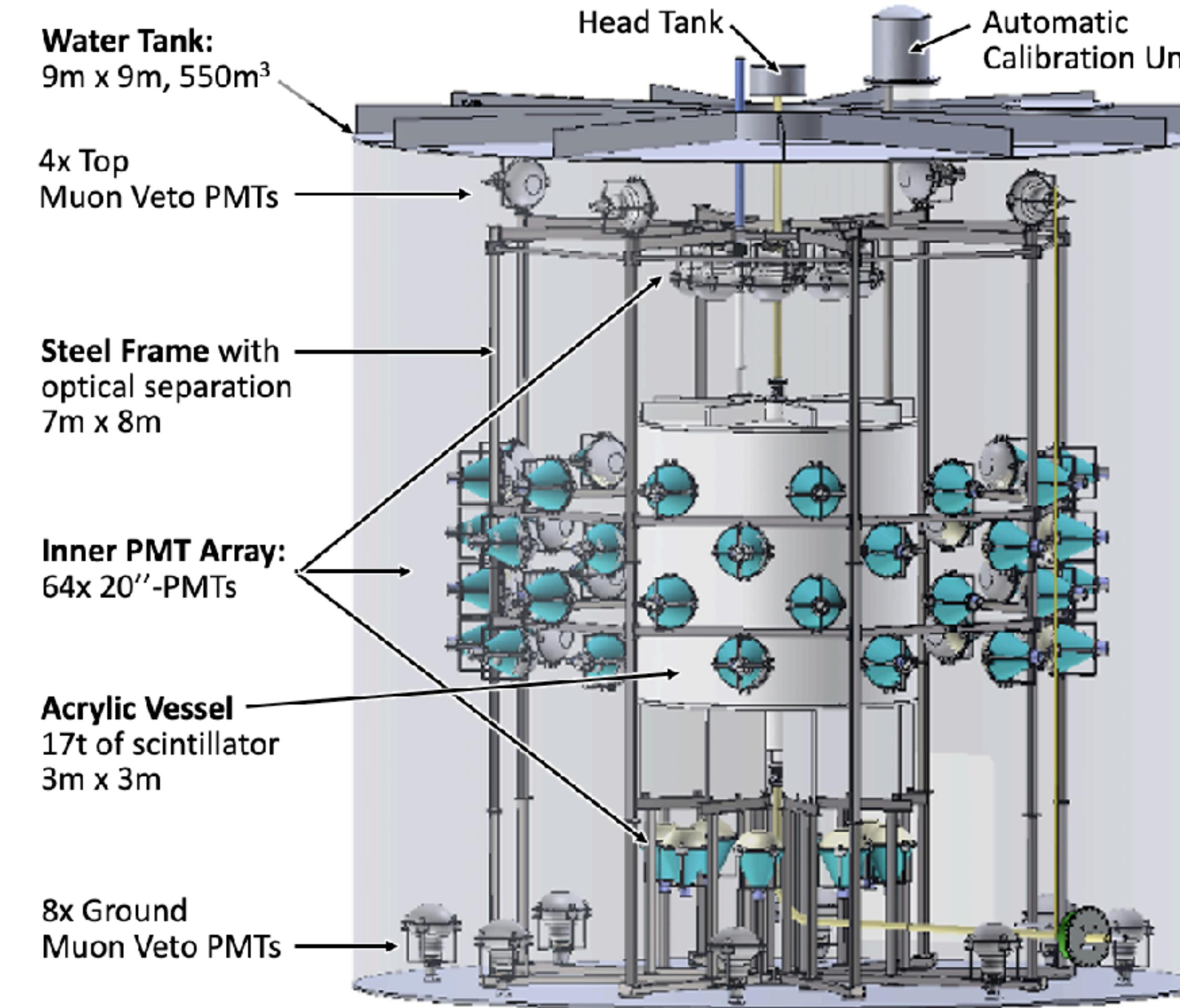
A 20 ton detector to monitor LS radiopurity during purification plants commissioning and JUNO detector filling
