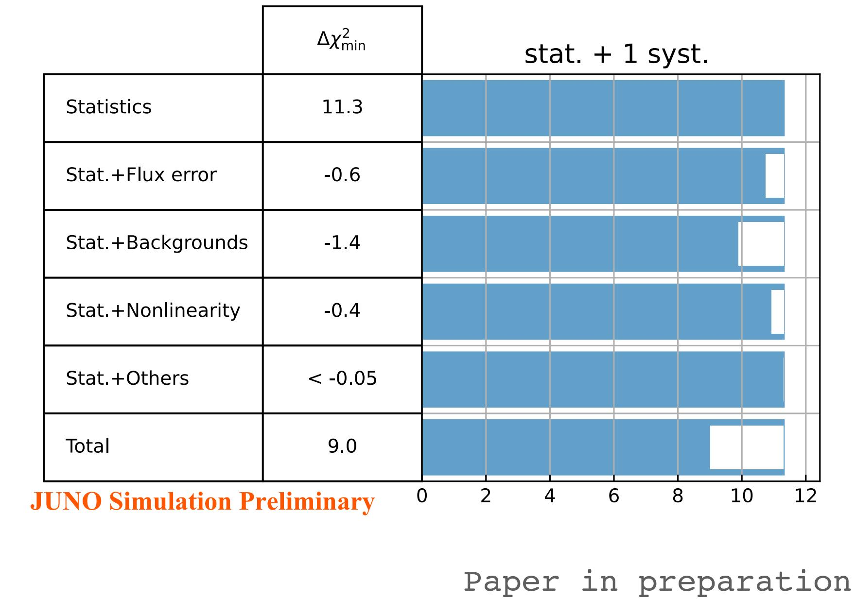
JUNO sensitivity on neutrino mass ordering: 3 $\sigma$  (reactor only) in  $\sim 6$ y with 26.6 GW<sub>th</sub>
