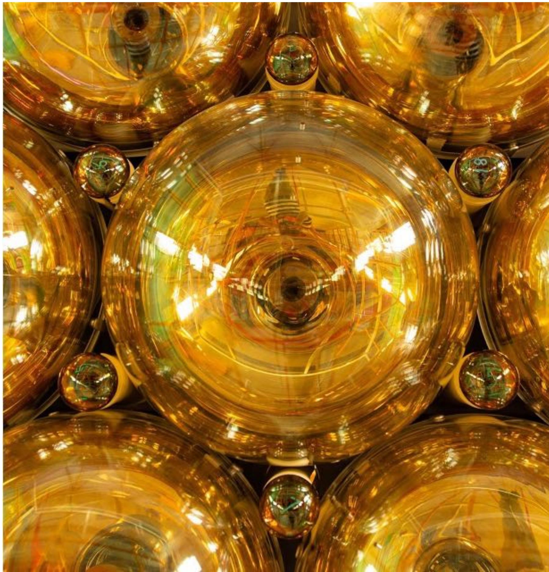
Clearance between PMTs: 3 mm
