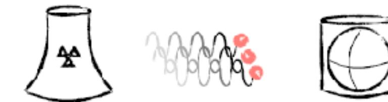
3  $\text{GW}_{\text{th}}$  reactor  $\rightarrow \sim 10^{21} \bar{\nu}_e/\text{s}$
