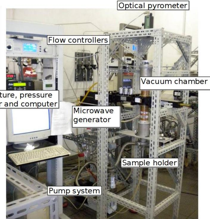
➤ **Diamond film is deposited by Microwave Plasma Enhanced Chemical Vapour Deposition (MWPECVD) on a commercial low-cost diamond substrate.**
