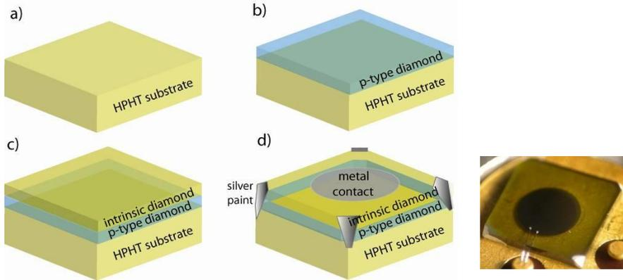
**Fabrication process of diamond detector operating in planar configuration**
