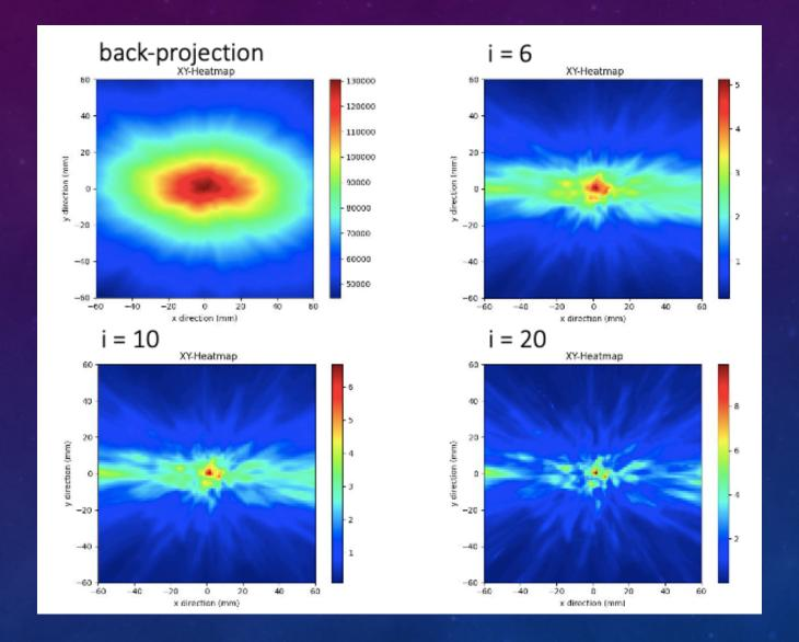
Spherical source, 1 cm diameter, phantom loaded by B10 (scatterer + emitter) 5:1
