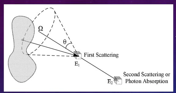
2 stage system: front plane SCATTER det. + back plane ABSORBER det.
