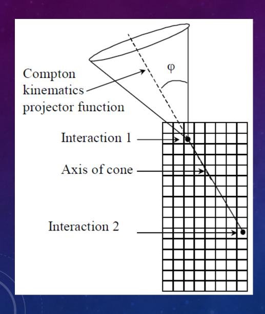
single stage Compton imager exploing 3D position sensing CZT
