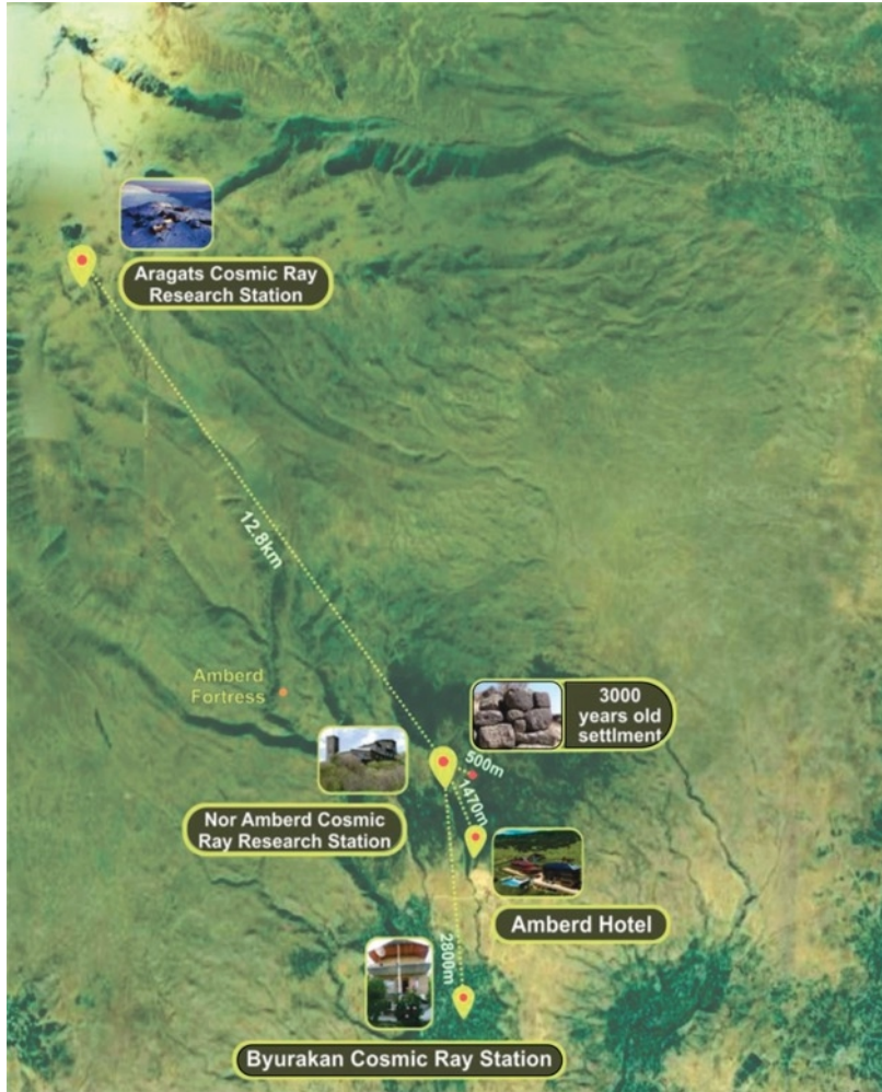
The map of networks of NaI spectrometer locations: five on Aragats (3200 m), one in Burakan (1700 m), and one in Nor Amberd station (2000 m). Electric mills and lightning locators are installed on Aragats (5 units) and in Nor Amberd.
