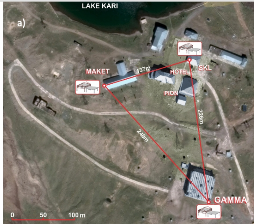
The map of Aragats station with STAND1 network; b) Stand1 unit: vertically stacked 1 cm thick, and 1 m 2 area plastic scintillators; c) Stand1 unit: stand-alone 3 cm thick plastic scintillator with the same area.
