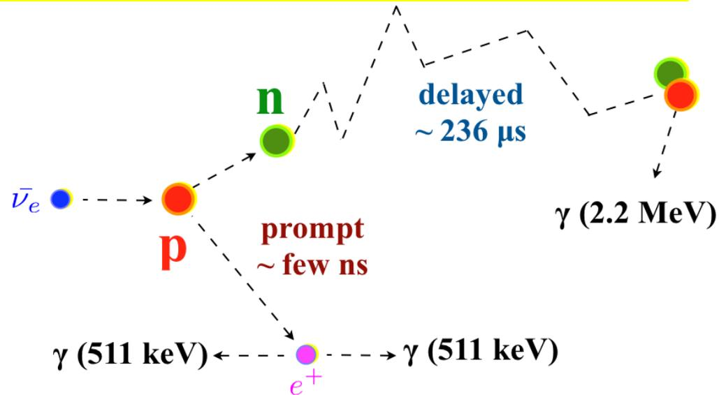
The time coincidence between the positron and the  $\gamma$  from the capture rejects the uncorrelated background
