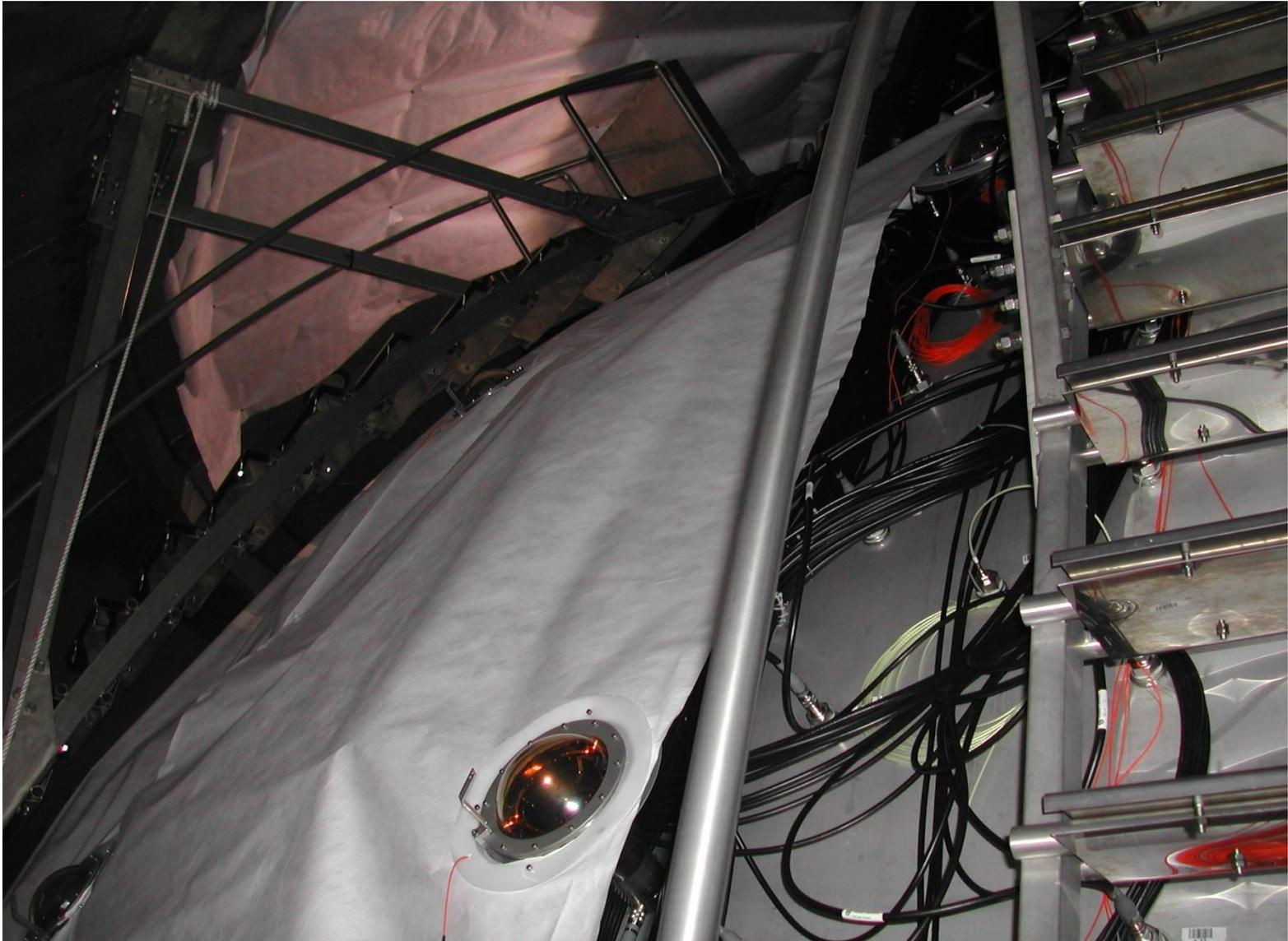
Tyvek on the surface of the Water Tank dome
