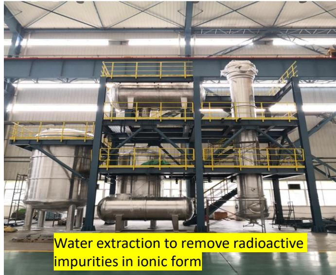
Water extraction to remove radioactive impurities in ionic form
