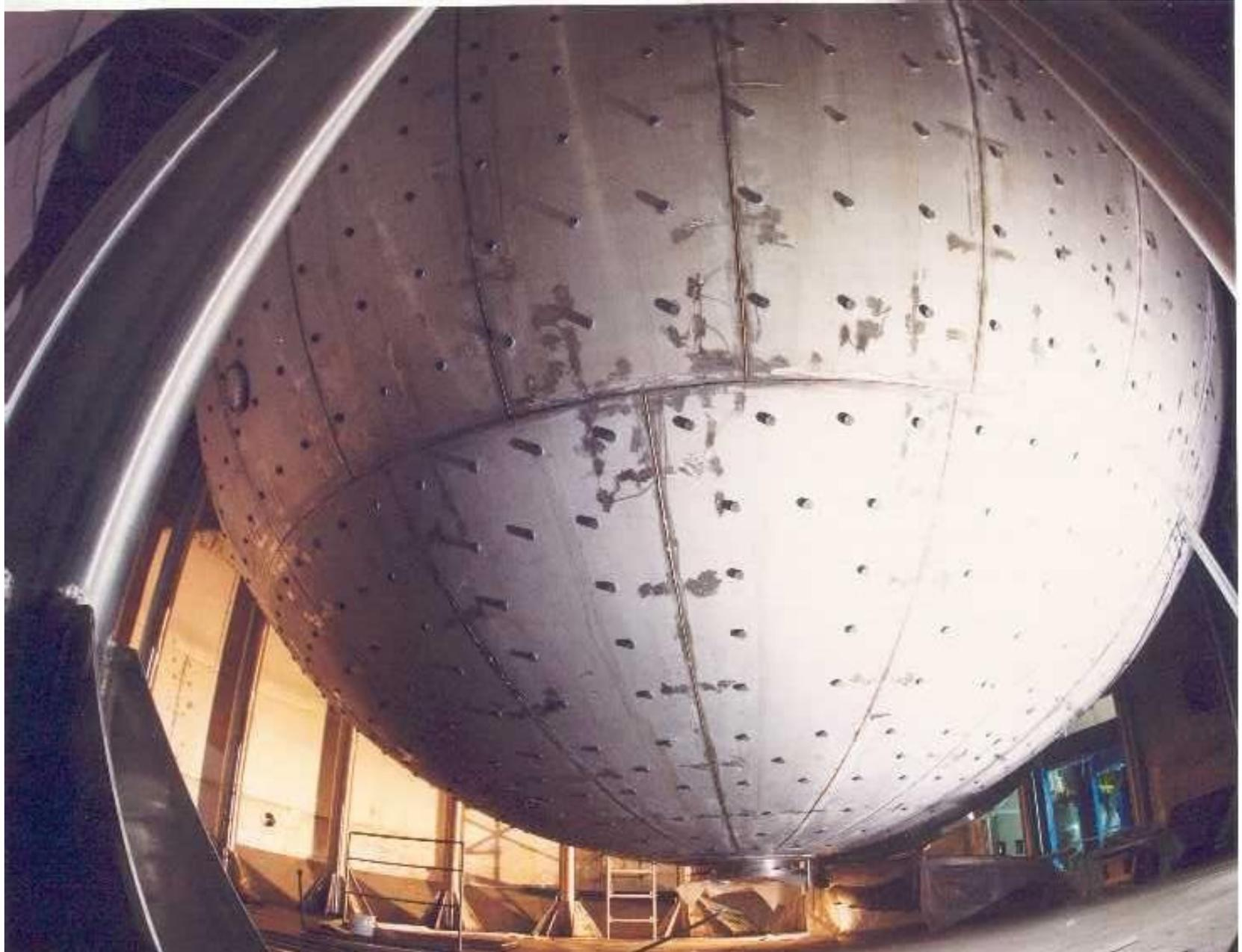
PMT's on the sphere surface
