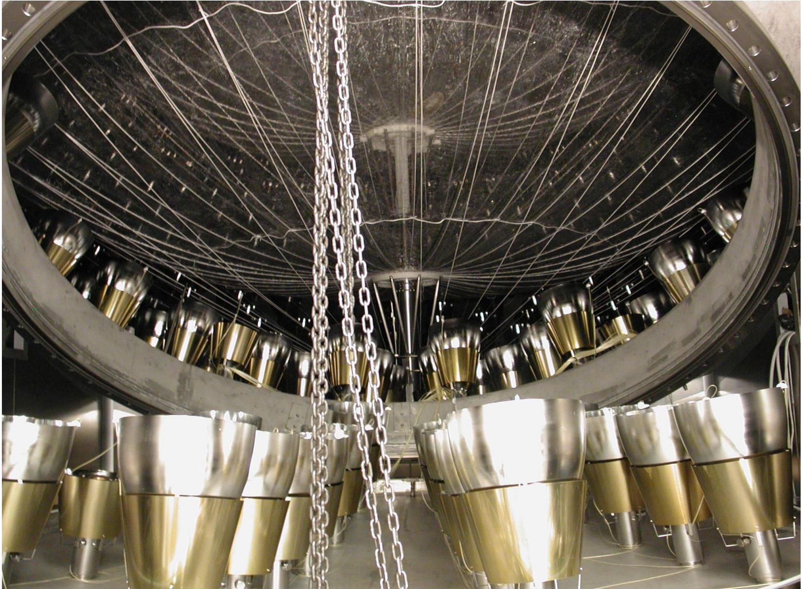
Muon veto: tyvek (diffusive panels) and phototubes on the external sphere surface
