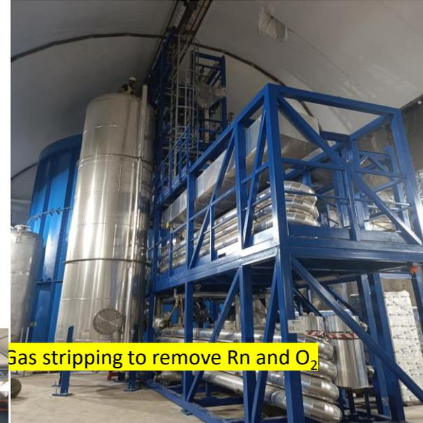
Gas stripping to remove Rn and O<sub>2</sub>
