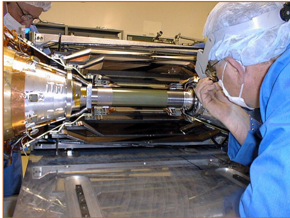
Silicon Vertex Tracker of BaBar at SLAC
