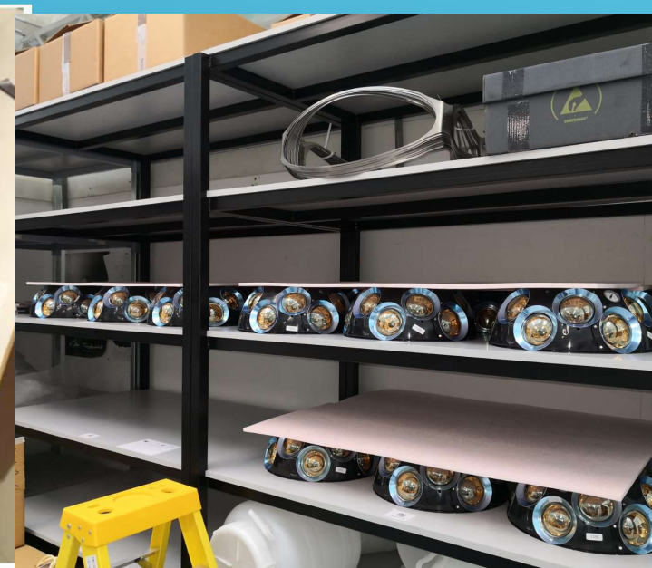
PMTs after integration in the mechanical structure
