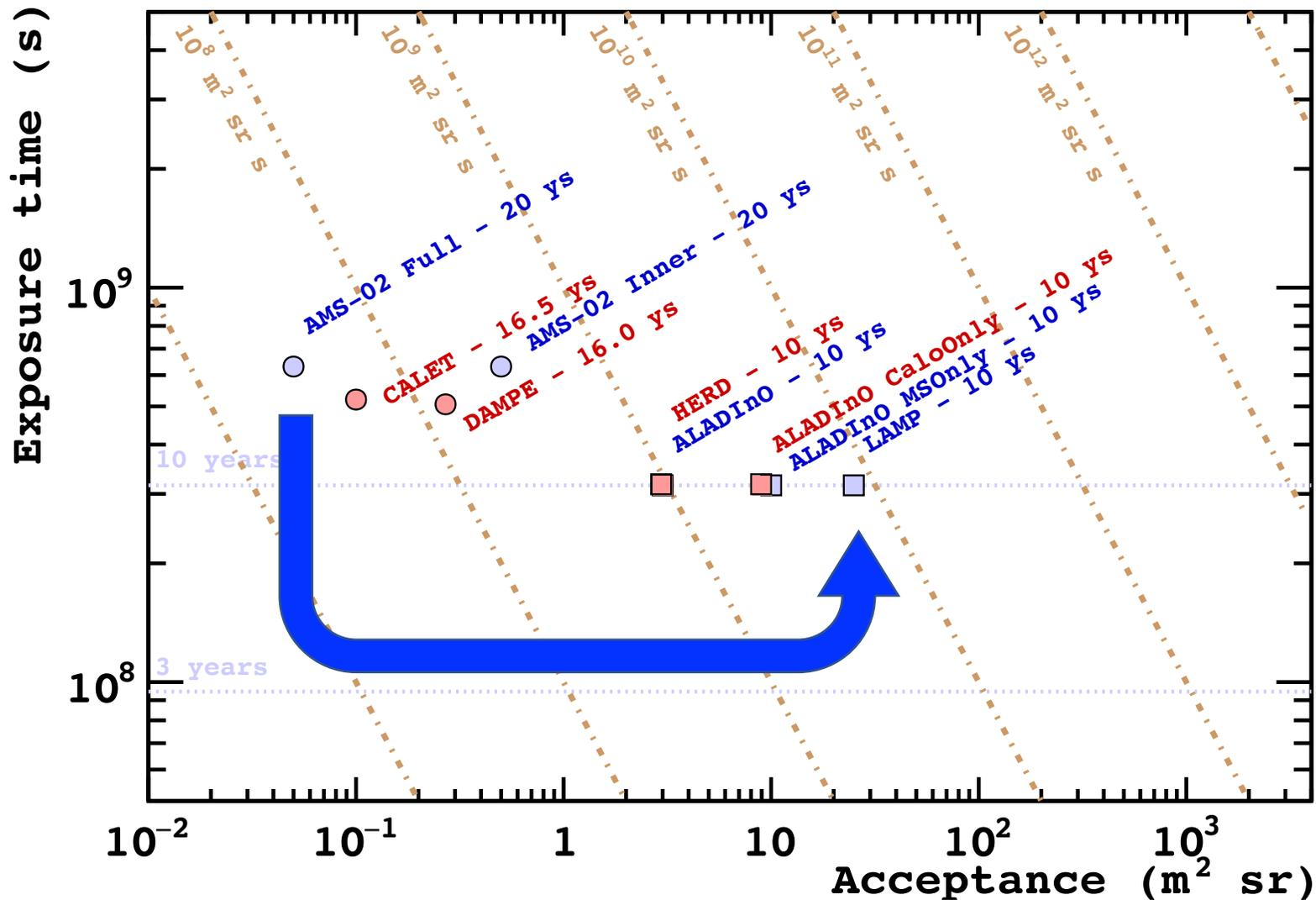
LAMP maintains the geometry of ALADInO, but focuses on nuclear antimatter. It features increased acceptance for the magnetic spectrometer and auxiliary detectors (TOF, Cherenkov), saving mass with a calorimeter-free approach. More than a factor of 30 is gained in acceptance over AMS-02.
