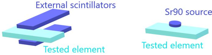
**Figure 6.16** Schematic example of PSD element testing using CR muons (left) or radioactive source (right)
