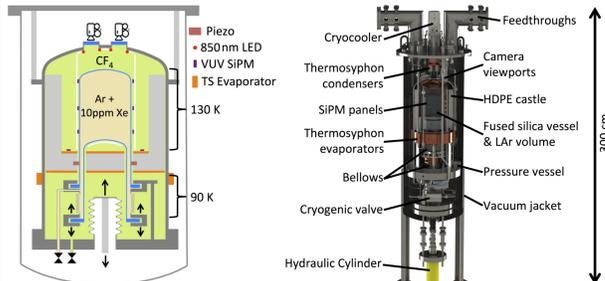
Schematic (left) and annotated solid model (right) of the SBC-LAr Detector.
