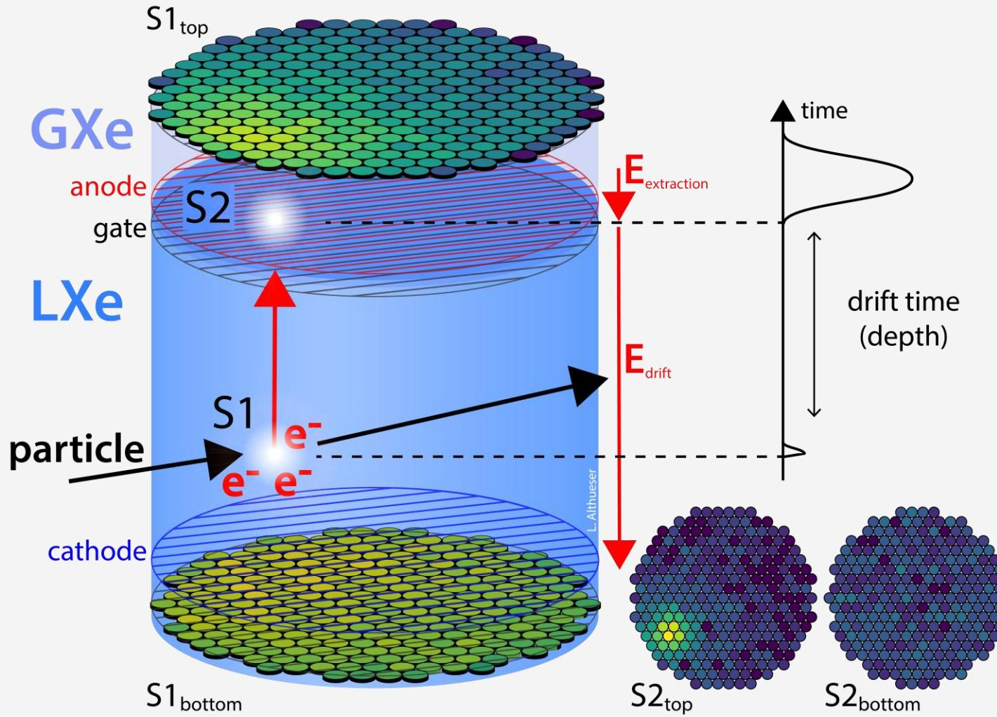
Working principle of dual-phase liquid noble gas time projection chambers (TPCs)
