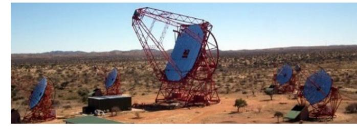
• H.E.S.S. phase II: 28m telescope; FoV 3.5°; first light 2012
