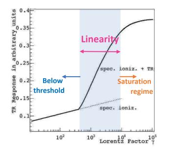
Linearity for  $10^3 < \gamma < 10^4$ · Electrons: 0.5 GeV  $< E_e < 5$  GeV
