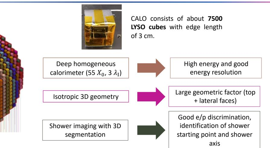
Each cube is readout by 2 systems. The double read-out system allows for **redundancy**, **independent trigger**, **and cross calibration** in order to reduce the systematic uncertainties (especially on the absolute energy scale).
