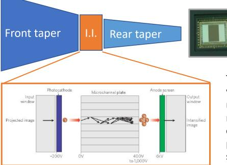
The **image intensifier** converts weak light signals into electrons, multiplies the electrons using a micro-channel plate, and then converts the electrons back into photons using a phosphor screen.
